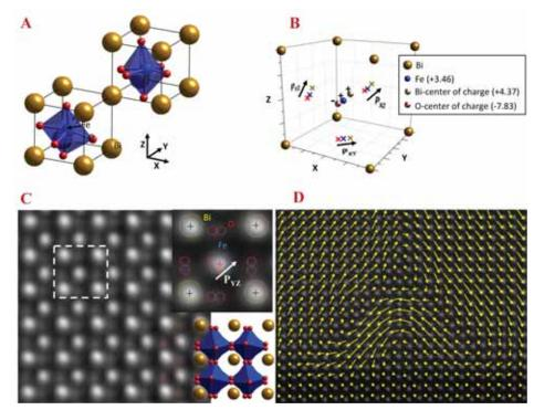
Figure 1: A. Crystal structure of BiFeO<sub>3</sub>. B. The projection of electric dipole moment and atoms in a unit cell of BiFeO<sub>3</sub>. C. The phase component of the electron exit wave determined from a TEM focal series. D. The two-dimensional map of local polarization in BiFeO<sub>3</sub> showing the existence of a polarization vortex.
