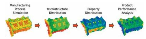
An illustration of the flow chart for an integrated computational materials engineering (ICME) toolset for an automotive engine cast aluminum cylinder head.
